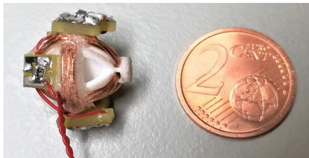
Figure 2 Miniaturized receiver compared to a 2-euro cent coin
