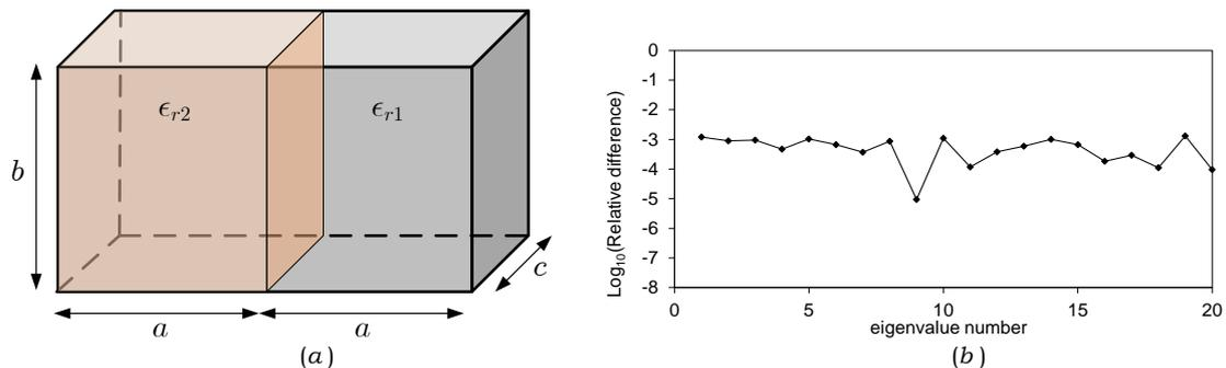
**FIG. 6** –Half-filled rectangular cavity: (a) Geometry of the structure ( $a = 5$  mm,  $b = 1$  mm,  $c = 10$  mm,  $\epsilon_{r1} = 1$ ,  $\epsilon_{r2} = 2$ ); (b) Relative difference between the present method and the results given by HFSS on the first 20 modes.
