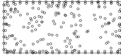
**FIG. 1** – WR90 rectangular waveguide (22.86\_10.16 mm<sup>2</sup>) and the collocation points used for the analysis by the variational meshless method.
