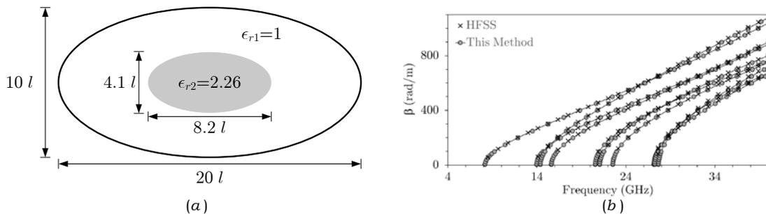
**FIG. 5** – Elliptic inhomogeneous waveguide. (a) Geometry of the structure ( $l = 1$  mm). (b) Dispersion diagram calculated by the variational meshless method (gray circles) compared with the HFSS simulation (black cross).
