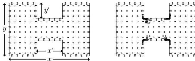
**FIG. 3** –Double Ridge Waveguide ( $x=30\text{mm}$ ,  $y=20\text{mm}$ ,  $x'=10\text{mm}$ , and  $y'=6\text{mm}$ ) and the collocation points used for the analysis by the variational meshless method before and after the refinement.
