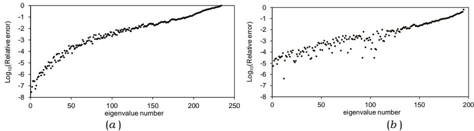
**FIG. 2** – Error in the calculation of the cut-off frequency of a WR90 rectangular waveguide by the variational meshless method with 248 collocation points: (a) TE modes; (b) TM modes.
