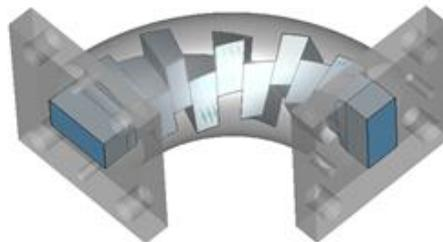
**Figure 1: Integration of a low-pass filter, a twist and a H-plane bend**
