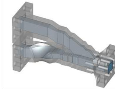
**Figure 2: Integration of an OMT with a twist****Table 2: Measured RF performances of the OMT with integrated twist**
