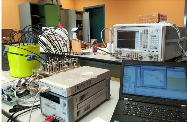
Figure 1. Overview of the realized microwave brain scanner.
